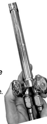
The torch body controls the gas output and connects the torch to the hoses. Always hold the torch body so that the torch valves are facing towards you, with the "Fuel" (acetylene) valve to your left and oxygen valve to the right.
